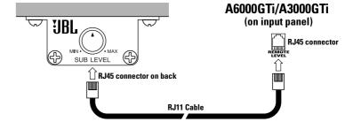
**Figure 1.** Connecting the Remote Level Control.
